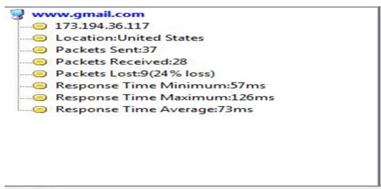
Fig. 11. Colasoft Capsa packet loss
