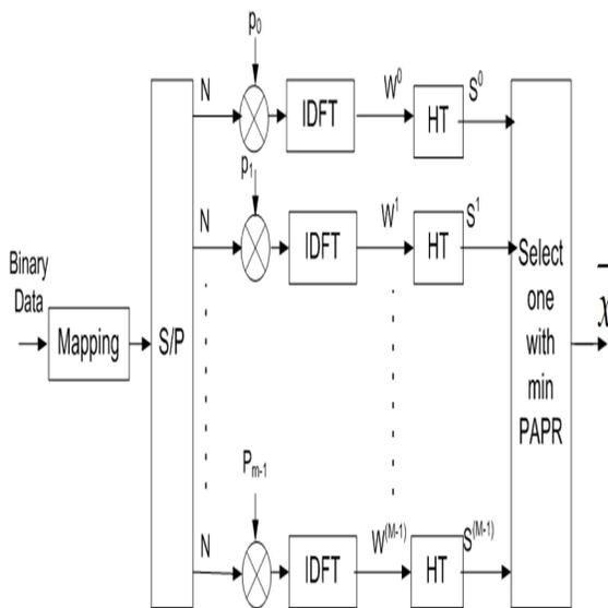
Fig. 2. Block diagram of Modified SLM with Hadamard Transform
