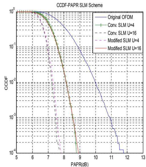
Fig. 4. Comparison of PAPR with SLM and Modified SLM
