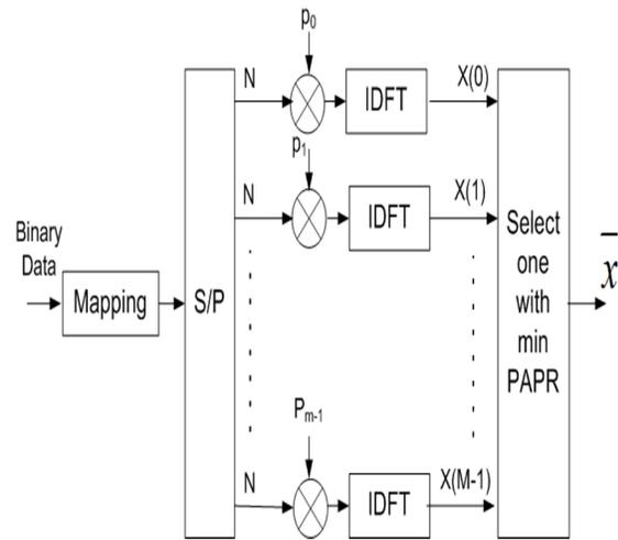
Fig. 1. Block diagram of conventional SLM technique
