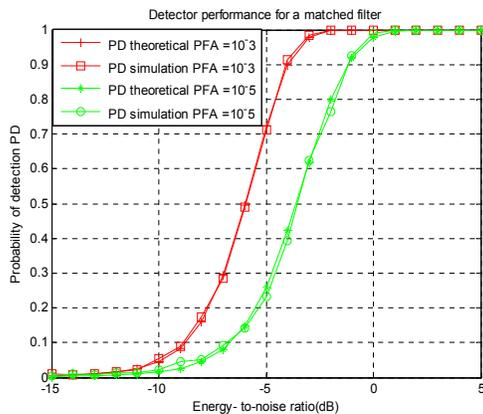
Fig. 2. Detection performance of matched filter
