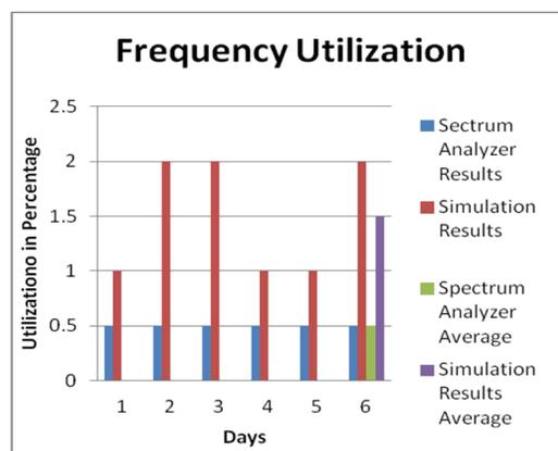
Fig. 4. Average utilization of band 400-600 MHz
