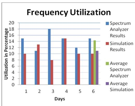
Fig. 2. Average utilization of band 50-250 MHz
