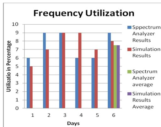
Fig. 3. Average utilization of band 250-400 MHz
