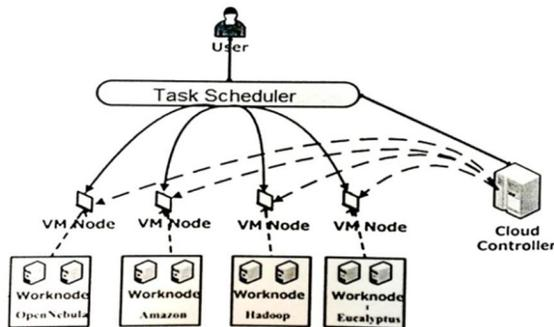
Fig. 1. The framework of a scheduling system in cloud computing environment.
