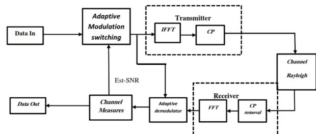
Fig. 5. Illustrate the Block diagram of AMC system.
