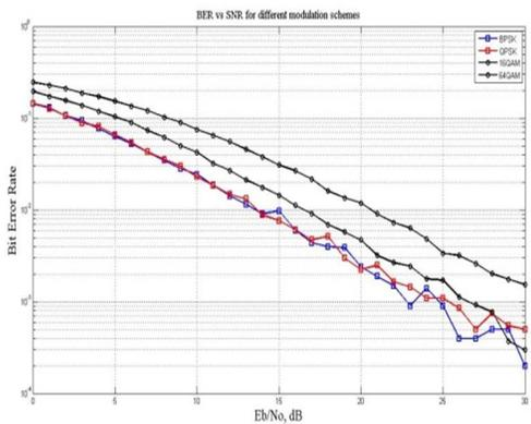
Fig. 8. BER vs.  $E_b/N_0$  over Rayleigh channel without using OFDM
