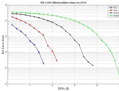
Fig. 7. BER vs.  $E_b/N_0$  over AWGN channel without using OFDM
