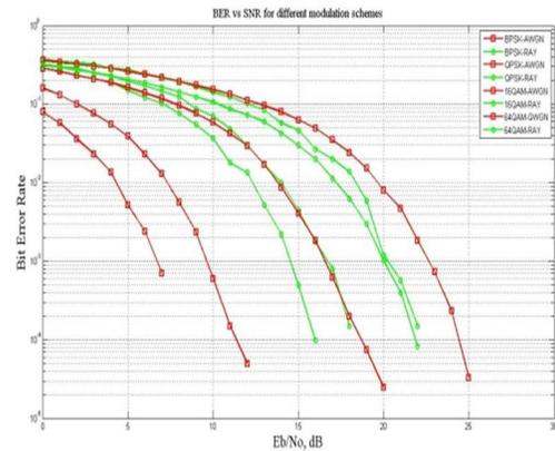
Fig. 9. BER vs.  $E_b/N_0$  over AWGN and Rayleigh channels with using OFDM
