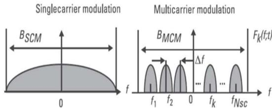
Fig. 1. SCM and MCM frequency spectra.
