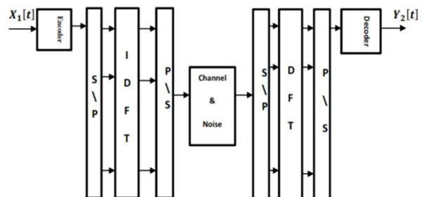
Fig. 3. Discrete time baseband equivalent model of an OFDM system.
