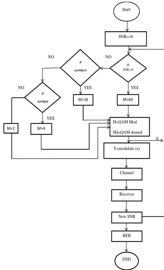
Fig. 6. Illustrate the flow chart of AMC simulation system.
