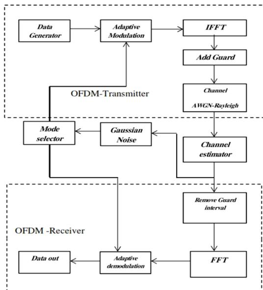
Fig. 4. Illustrate the Block diagram of OFDM adaptive modulation system.
