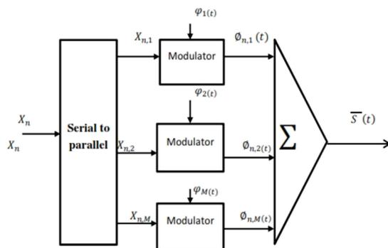
Fig. 2. Multi Carrier Modulation Block diagram
