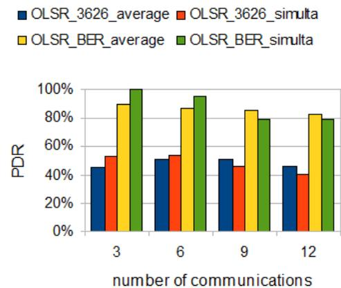
Fig. 7. Multi-communication impact on BER-OLSR PDR and compared with standard OLSR.
