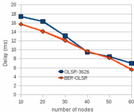
Fig. 3. Evolution of Transmission Delay According to the Number of Nodes in Fixed Scenario.
