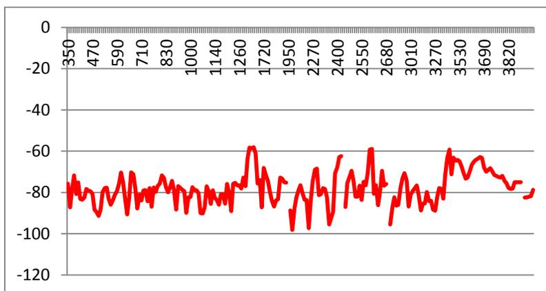
Fig. 6. The relationship between distance and Rx-Qual in this cell.
