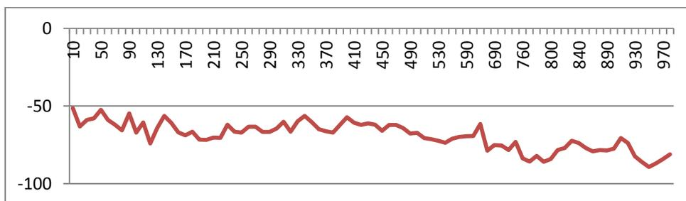
Fig. 2. The Relationship Between Distance And Rx-Qual In This Cell.
