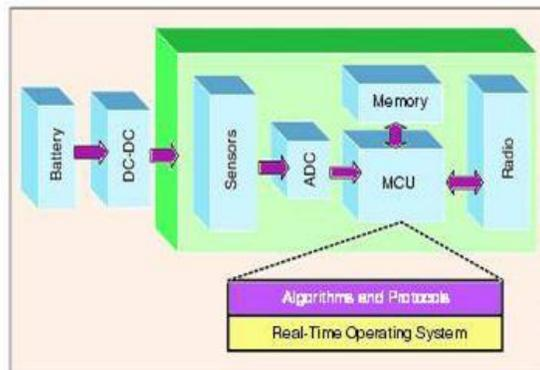
Fig. 2. System structure of a wireless node sensor
